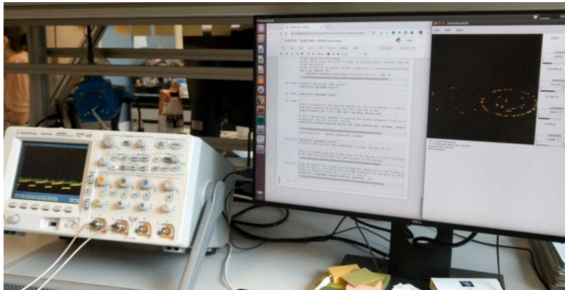
Figure B.3.: CTXCTL being used to configure a SNN , including parameters, input connections, and multi-layer connectivity schemes, implemented using a Jupyter Notebook for Python. The Jupyter Notebook can be used together with CTXCTL as a server option is made available. The oscilloscope on the left shows analog and digital measurements from the neurons on the chip that can be configured using the same setup.
